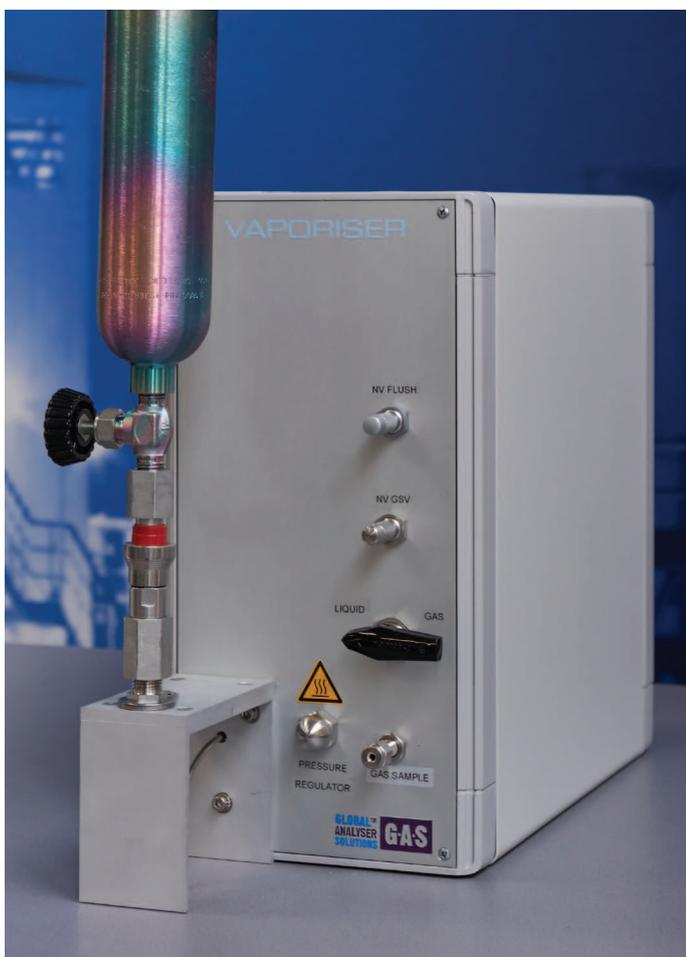
Figure 2. Vaporiser with mounting support for cylinder
