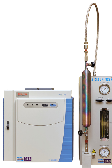
Figure 7. Refrigerants analyser using LSV and Sample Securitiser
