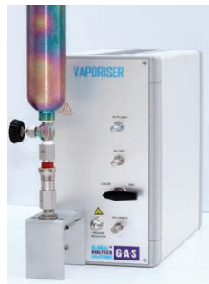
Figure 7. Vaporiser for injecting LPG as a gas
