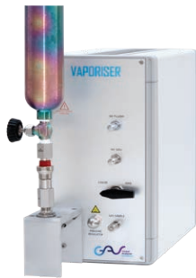
Figure 7. Vaporiser for injecting LPG as a gas
