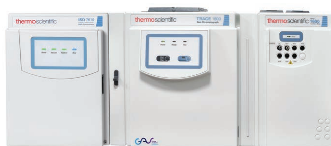
Figure 2. GC 1600 with valve oven and ISQ 7610 mass spectrometer with and AEI source (Advanced Electron Ionisation).
