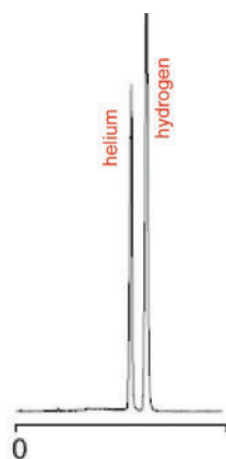
Figure 5 helium and hydrogen on TCD (N 2 or Ar carrier gas)
