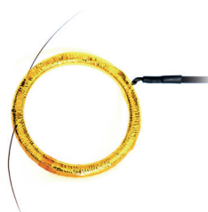
Figure 3. Capillary column with resistive heating provides fast heating rates and short run time.
