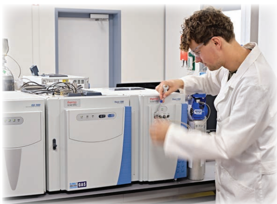
Figure 5. Extended gas analyser equipped with TCD, PDD and mass-spectrometer (ISQ-7000) for analysis of ammonia and many other species.
