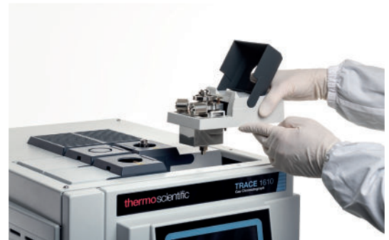
Figure 5 Swift exchange of injector and detector
