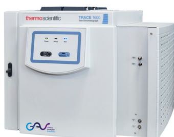
Figure 2 Low-level ammonia analyser on Thermo Trace GC1600
