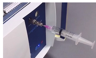
Figure 2 Vacuum sampling from a single syringe (above) and autosampler for multiple syringe injection (right).
