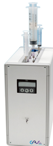
Figure 2 Vacuum sampling from a single syringe (above) and autosampler for multiple syringe injection (right).
